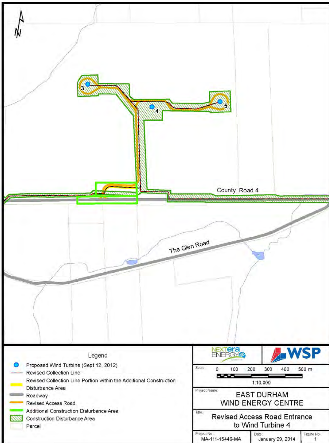
Figure 1: Revised Access Road Entrance for Turbine 4
