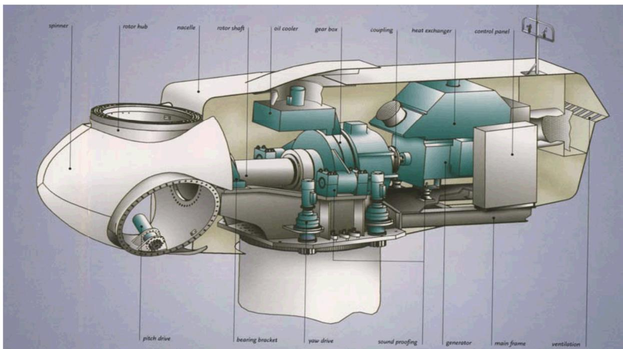
Figure 1: GE Energy 1.6-100 wind turbine nacelle layout
